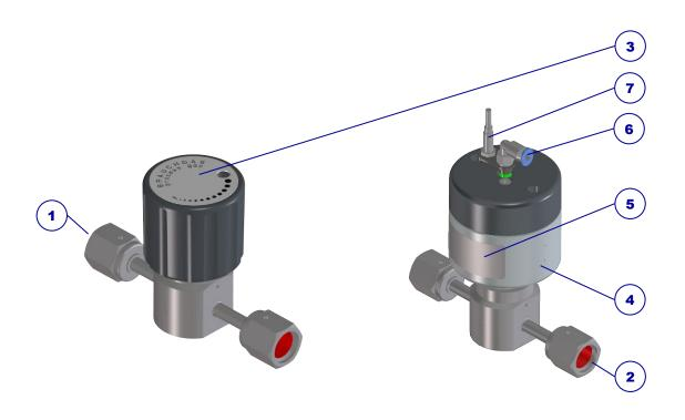
Illustration 1: Diaphragm valve design MV3-VCR
